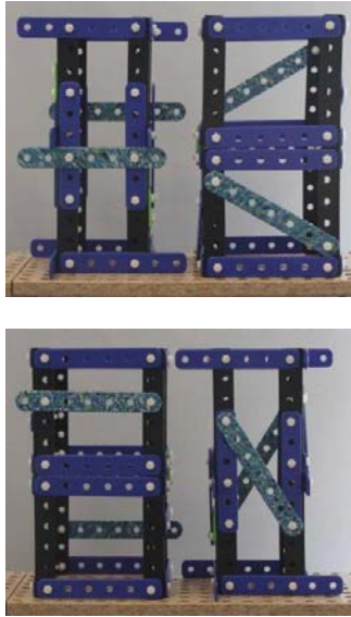
Figure 1b: Low Alignability condition: unstable model on left, stable (braced) model on right, showing the two counterbalanced versions
